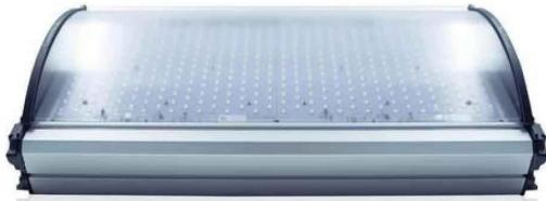
The Maxi Xion 384 F2 is designed and manufactured in France, it is solid, watertight (IP52) and resistant with an aluminium body and a slightly frosted polycarbonate diffuser for the perfect balance between performance and absence of glare. It is available with several colour temperatures (4000K, 5000K, 3000K optional), power supplies and dimming/radio control systems.
