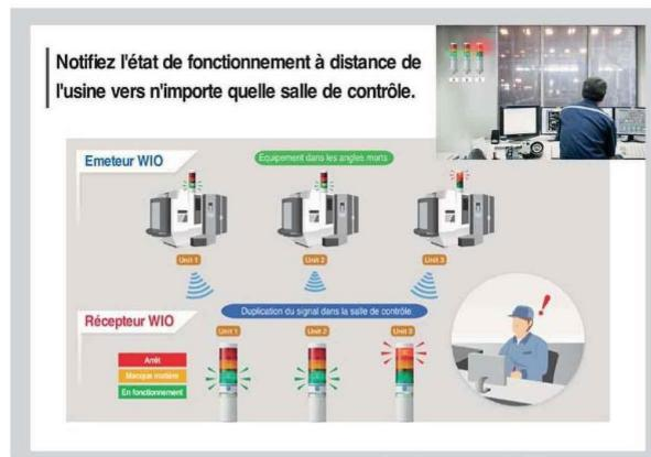
solution. It provides a visual representation of the status of installations, even if they are distant or out of sight, there is no need for cables, it uses reliable wireless communication system with a reach of up to 400m thanks to its long distance Bluetooth technology.
